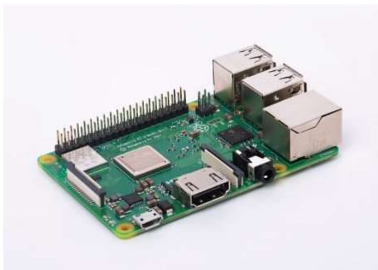
Figura 13. Raspberry Pi model B+ Fuente: (Raspberry ORG, 2018)
