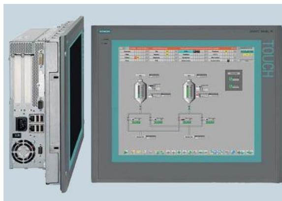
**Figura 12.** Simatic HMI panel
