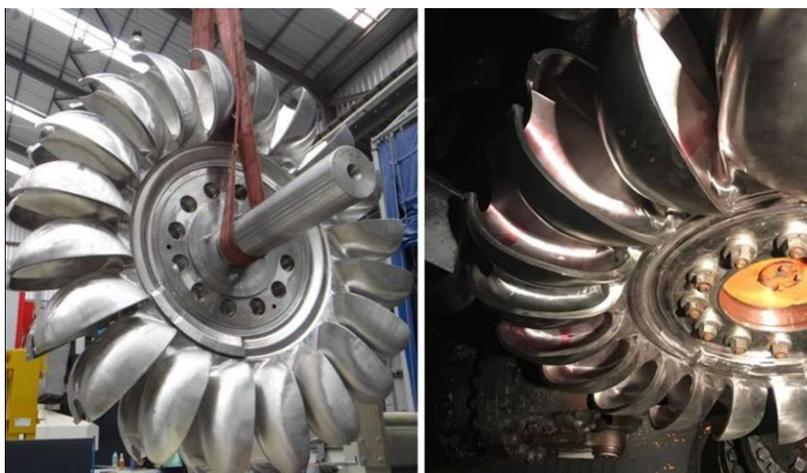
**Figura 13.** Turbina Pelton - Central Pucará
