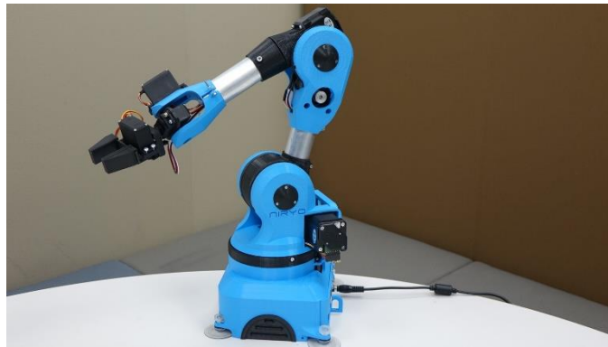
Figura 1. Niryo One. Robot open source de 6 grados de libertad
