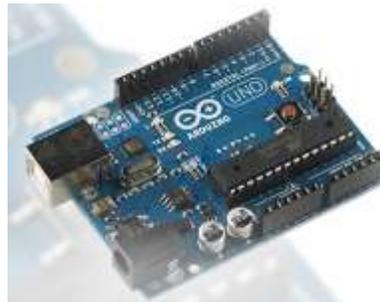
**Figura 28 Tarjeta Arduino**
