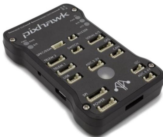
**Figura 32.** Tarjeta Ardupilot Pixhawk
