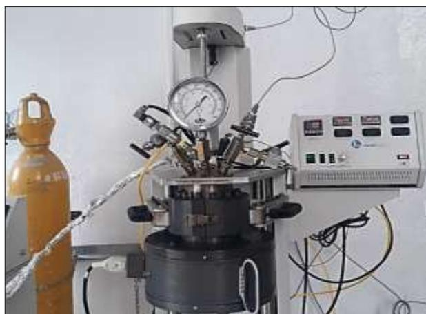
*Figura 9.* Reactor Batch Parr Instrument 4575
