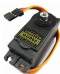
**Figura 30.** Servomotor MG995
