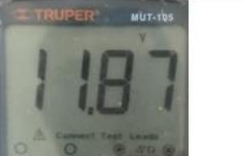
A digital multimeter (TRUPER MUT-105) displaying a voltage reading of 11.87V. The display is in green and shows a 'V' symbol above the digits. Below the display, there are several small icons and text including 'Connect Test Leads'. |
