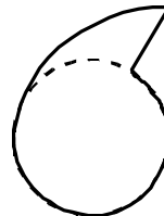
Cam profile with abrupt transitions
