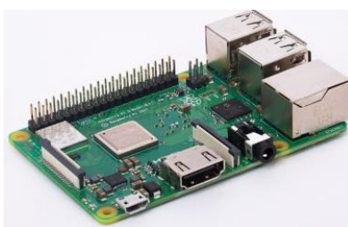
Figura 28. Raspberry pi 3 B+ Fuente. (Raspberry Pi Foundation, s/f)
