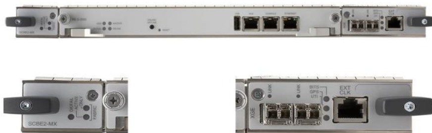
Figura 32. Switch Control Board (SCBE2) - Juniper MX480
