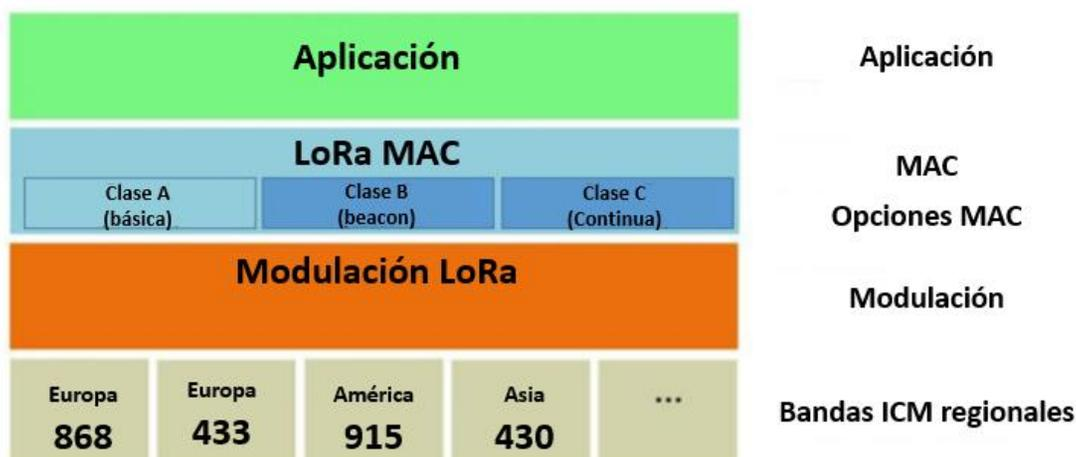
**Figura 8.** Capas LoRaWAN.
