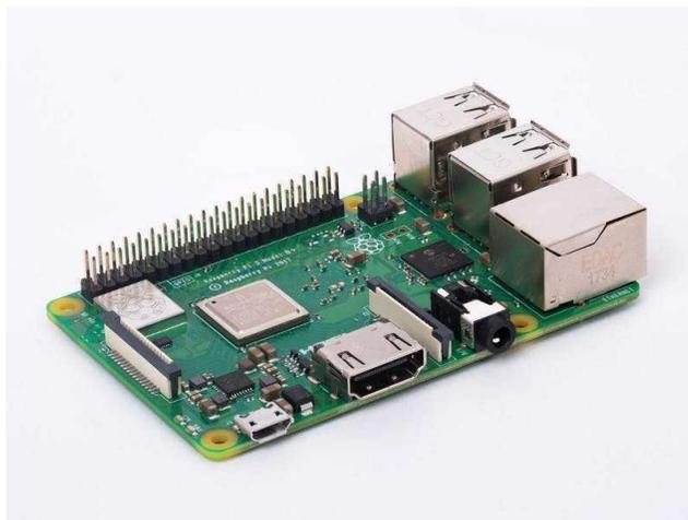
**Figura 6.** Raspberry Pi 3 Modelo B+
