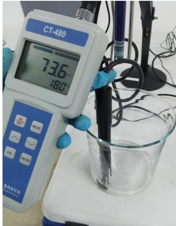
**Figura 14.** Conductímetro Marca Boeco Germany, Modelo CT-480
