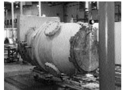
Model 810 undergoing hydrostatic testing
