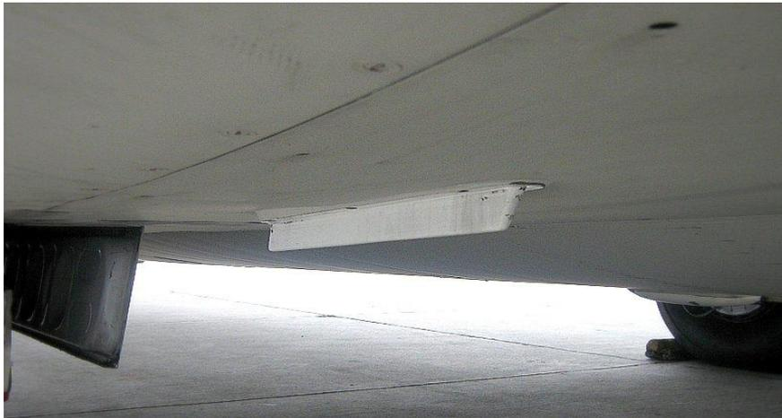
**Figura 2.26:** Antena Marker Beacon
