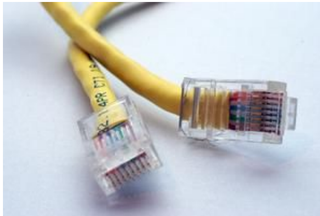
Figura8. Conector RJ45, cable UTP Cat. 5
