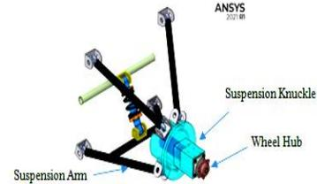
Figure 2. Suspension System and its main parts
