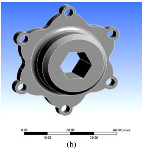
Figure 4. Topological Analysis of the Wheel Hub: (a) Original part, (b) Optimized part
