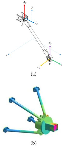
Figure 7. Suspension Arms: (a) Force Diagram, (b) Equivalent Stress Simulation
