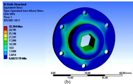
Figure 3. Wheel Hub Analysis: (a) Force Diagram , (b) Equivalent Stress Simulation
