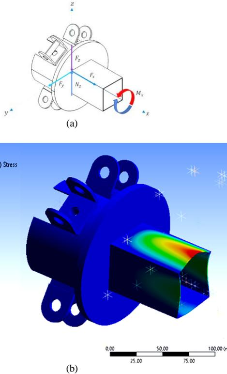
Figure 6. Suspension knuckle Analysis: (a) Force Diagram , (b) Equivalent Stress Simulation
