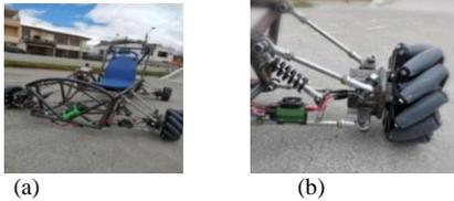
Figure 8. The Omnidirectional Vehicle: (a) All of Systems, (b) Suspension System
