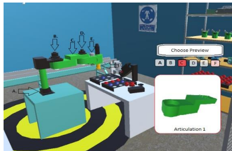
Fig. 7. Morphology of the SCARA robot manipulator
