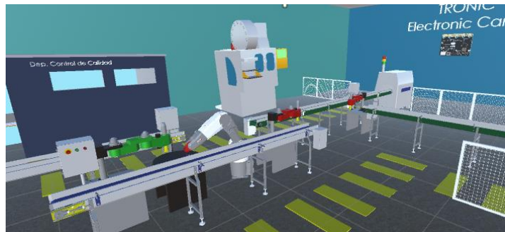
Fig. 9. Industrial process of electronic cards assembly
