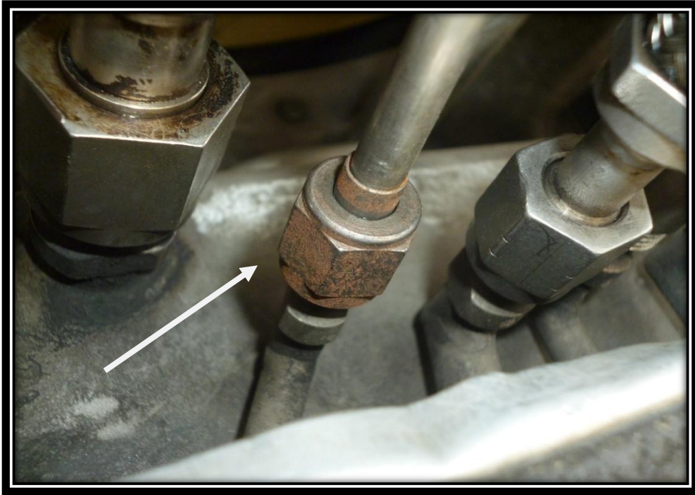
Figura 32: Water/ Methanol Shields drain tube
