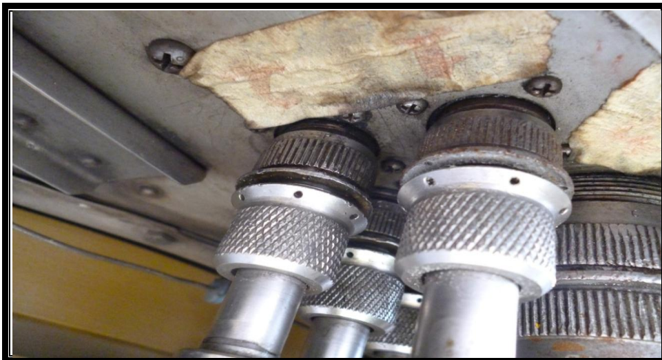
Figura 3.21: Conexión Cruise Pitch Lockc HUB SW.
