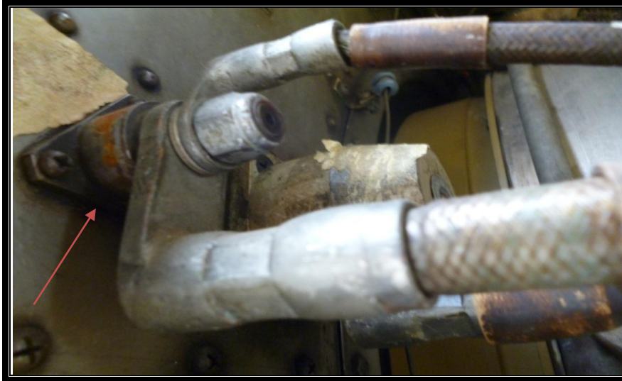
Figura 3.18: Conexión Started and feathering pump ground terminal
