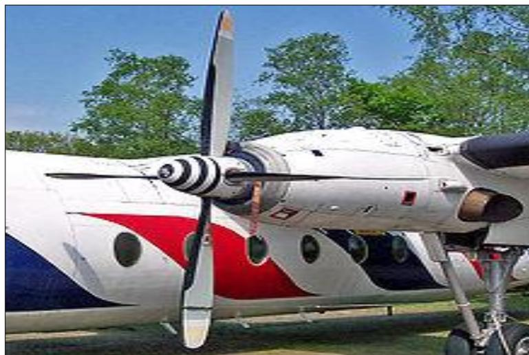
**Figura 18 Motor Rolls-Royce Dart RDa.7 Mk 532-7L**
