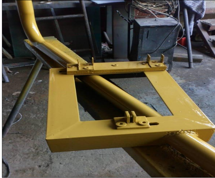
Figura 34 Herramienta Hoisting Cradle Assembly
