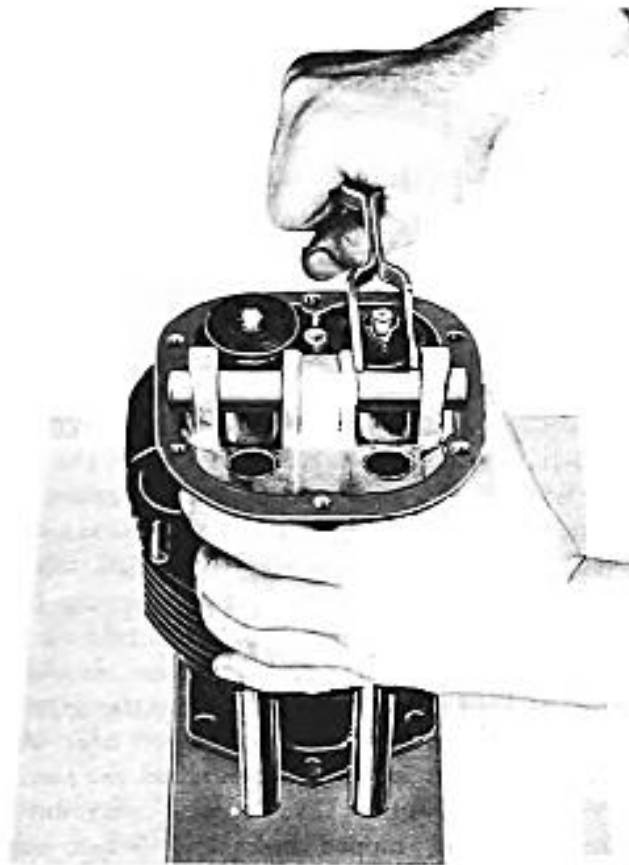
Figure 19. Compressing Valve Spring to Remove Locks
