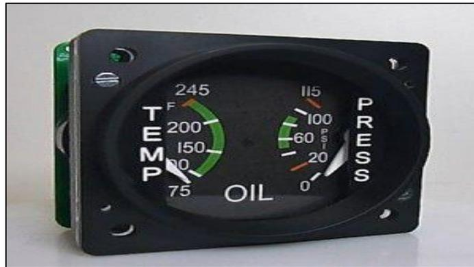
**Figura 49** Indicador combinado de Oil Temp and Oil Press
