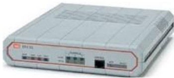
PADS ( Packet Assembler/Disassembler )
