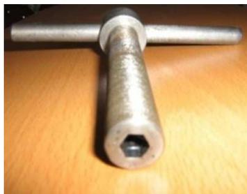
Figura.3.30 Punta hexagonal del tornillo extractor
