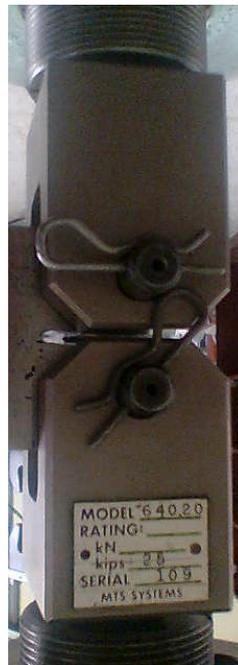
**Figura 3.5 Mordazas FRACTURE MECHANICS GRIPS Modelo 640.20**
