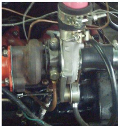
**Figura 3.1. Turbocompresor**
