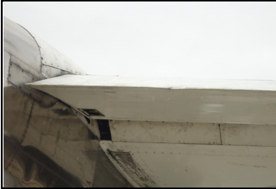
Figura 3.23: Flap exterior instalado
