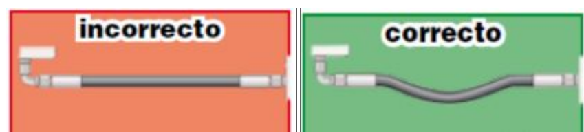
Figura 53 Instalación de manguera, influencias del ambiente Fuente: http://www.parker.com/parkerimages/Parker.com/Divisions-2011/Hose%20Products%20Division%20-%20Europe/Literature/Bulletin%20C4400-A_ES%202008-06-04.pdf
