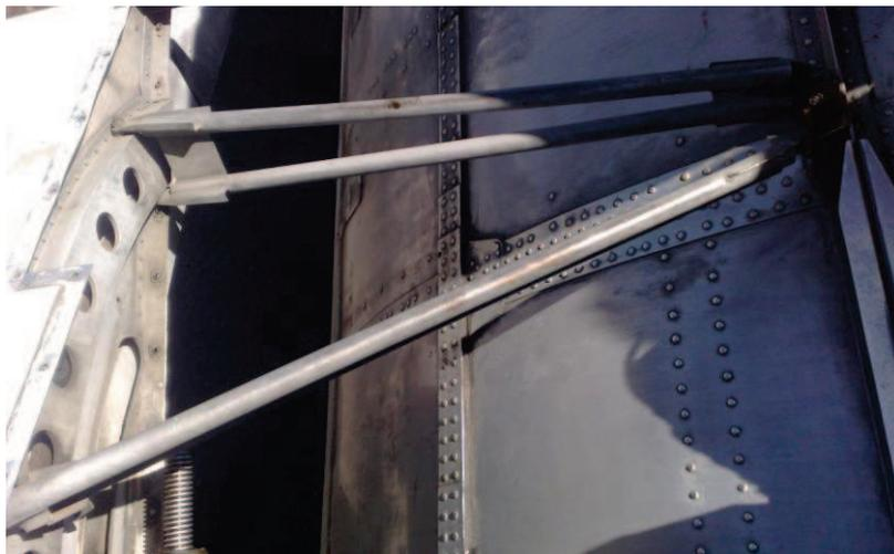
**Figura 3.35: Viga triangular**
