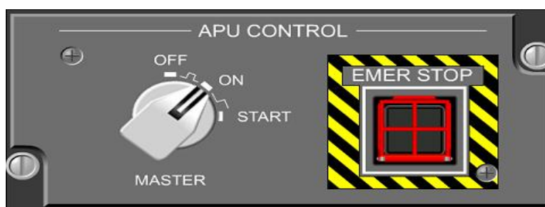
Figura 2.8. Panel de Control del Auxiliary Power United Fuente: Manual Embraer 170/190 Power Up and Power Down Procedures
