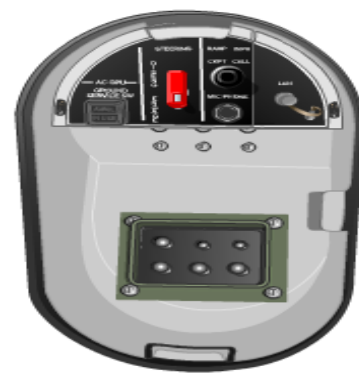
Figura 2.3. AC External Power Panel Fuente: Manual Embraer 170/190 Power Up and Power Down Procedures
