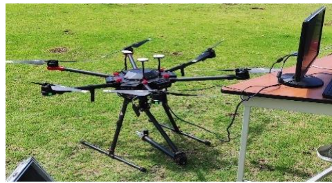
Figure 9. DJI Matrice 600 Pro UAV provided by the ARSI research group.
