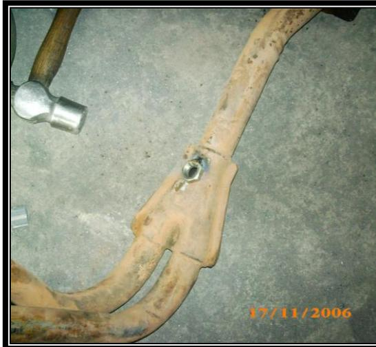
**Figura 3.47 Base del sensor HEGO adaptada**
