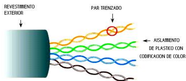
FIGURA No.1.75 Cable UTP
