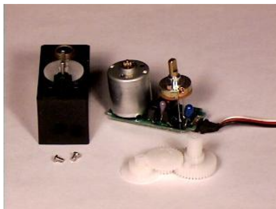
FIGURA No.1.56 Servomotor Centroid
