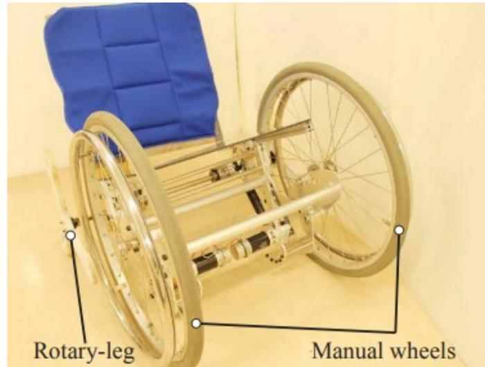
*Nota.* Tomado de Active Rotary-Legs Mechanism for Stair-Climbing Mobility Vehicle, por Sasaki & Suzuki, 2018, IEEE Robotics and Automation Letters.
