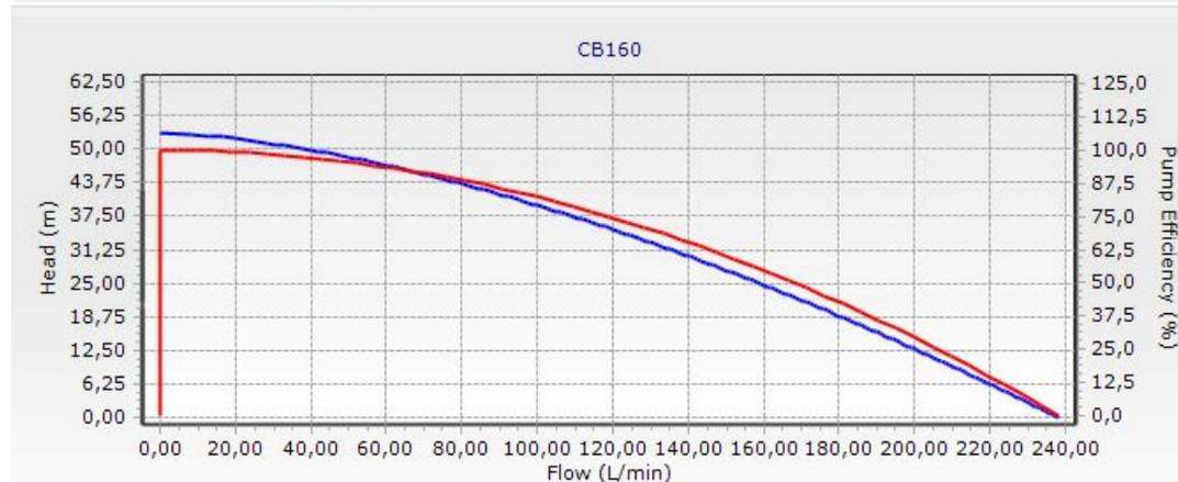
Coefficients: a = 52,99 m; b = 9,429e-003 m/(L/min)^c; c = 1,578
