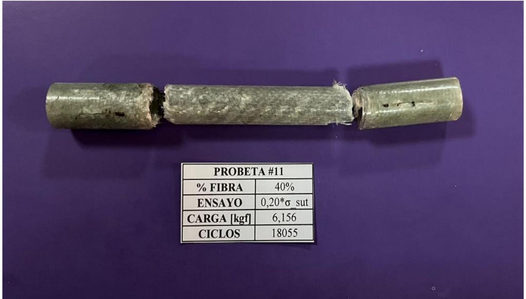
**Figura 18.** Rotura Probeta #11 – Vf=40%
