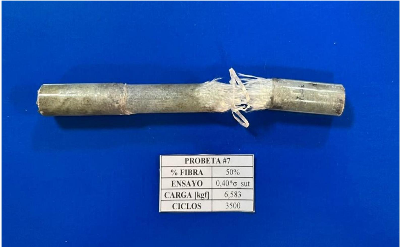
**Figura 17.** Rotura Probeta #7 – Vf=50%
