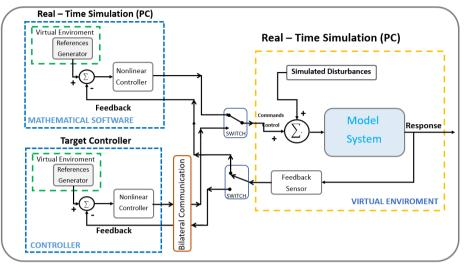
Fig. 2. Methodology for the control and visualization of industrial process
