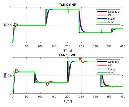
Fig. 10. Control actions of PID, Fuzzy and MPC controllers for tank 1 and tank 2
