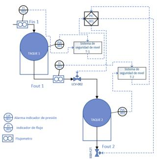
Fig. 1. P&ID diagram of the oxygen storage and distribution process.
