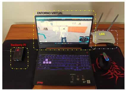
Fig. 8. HIL Implementation of the oxygen storage and distribution process
