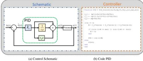
Fig. 5. PID Controller
