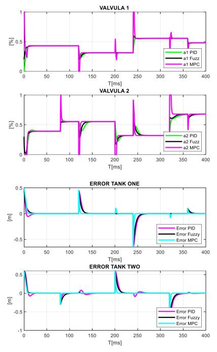
Fig. 11. Behavior of valves 1 and 2 And tank errors
