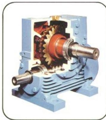
Figura 1.2 Motor Reductor
