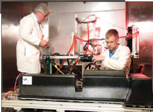
General Motors Battery Lab engineers prepare batteries for testing in the thermal chamber at the GM Tech Center in Warren, Mich.
