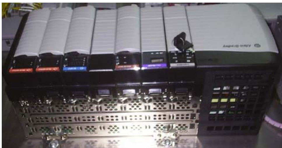
Figura 4. 3 PLC modular Allen Bradley
