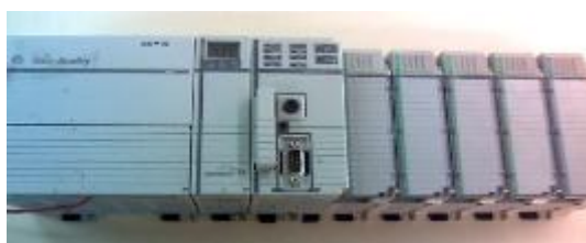
Figura 4.6 PLC 1768-L43 CompactLogix
