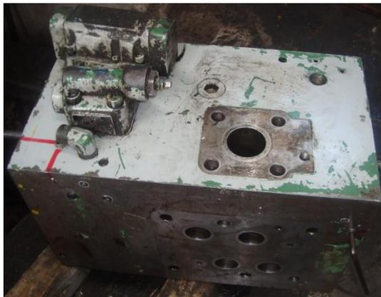
Figura 4.14: Bloque manifold principal
