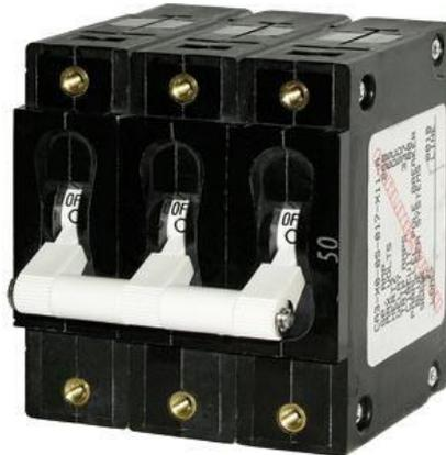
Figura 3. 27. Interruptor BlueSeatripolar C-Series 50[A], Icu 5[kA]<sup>251</sup>
