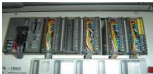
Figura. 7.1. PLC Modicon Compact CPU: 984-145.
