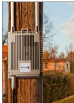
Figura 3.4.- Metro-Cell Outdoor 9364 1900-850MHz Alcatel-Lucent [E].
