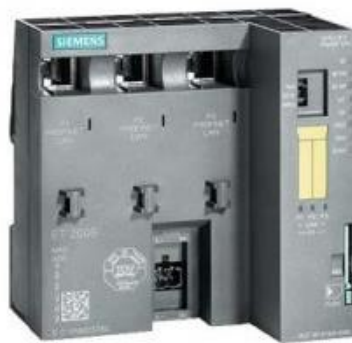
Figura 2.11: PLC SIMATIC ET 200S
