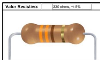
**Figura 4. 8. Resistor  $330\Omega$**
