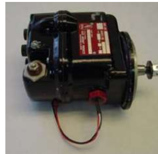
Figura 27. Sensor RPM instalado en el magneto (ADVANCED COMPANY, 2008)
